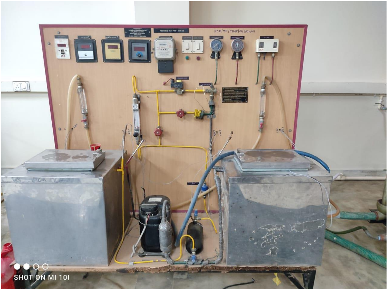
Fig:- Heat pump test rig
