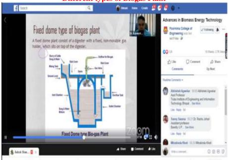
**Fixed Dome Type of Biogas Plant**
