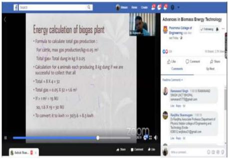
**Energy Calculation of biogas plant**
