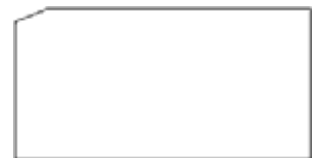
Chamfer with different distances
