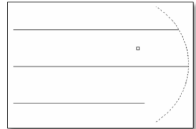
Lines Extended to an Arc (Arc is boundary edge)
