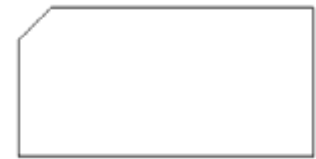
Chamfer with equal distances
