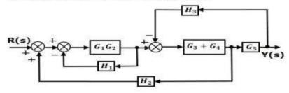
Step 2 - Use Rule 3 for blocks  $G_1G_2$  and  $H_1$ . Use Rule 4 for shifting take-off point after the block  $G_5$ . The modified block diagram is shown in the following figure.
