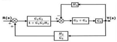
Step 3 – Use Rule 1 for blocks  $(G_3+G_4)$  and  $G_5$ . The modified block diagram is shown in the following figure.
