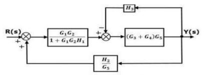
Step 4 – Use Rule 3 for blocks  $(G_3+G_4)G_5$  and  $H_3$ . The modified block diagram is shown in the following figure.
